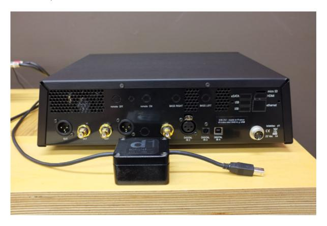
The main difference between the original total dac I reviewed and the d1-tube-mk2 DAC are the pair of ECC82/12AU7 dual triodes used in the output stage [footnote 2] instead of the discrete class A transistor circuit found in the D-1 dual DAC. The review sample also has the DSD option included so it can handle DSD64 (DoP), which the original D1 couldn't, as well as PCM resolutions to 24-bit/192kHz (Toslink input maxes out at 96kHz).
