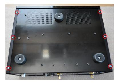
Remove 2 hexa screws on the rear panel of the server, they are shown in red on this photo:
