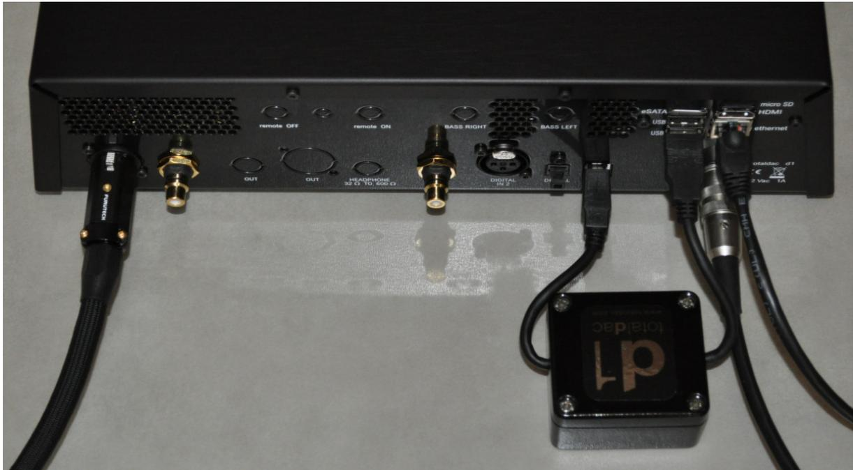
A USB cable/filter is used to connect the reclocker USB input to the embedded computer bottom USB connector.
